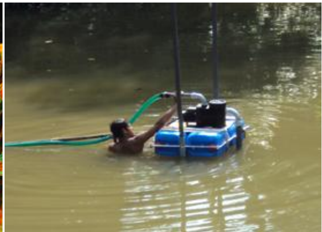
Solar Centrifugal Pump
